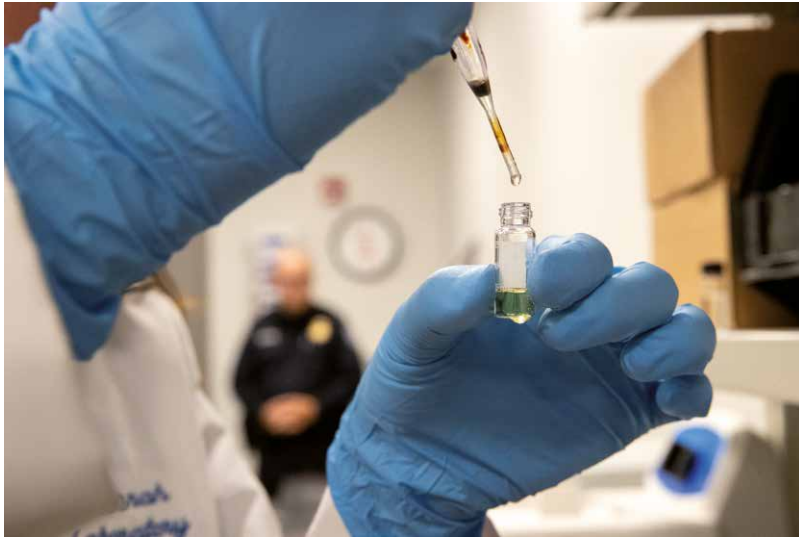
CBP scientist Shelby Stotelmyer adds a solvent to a suspected drug sample to extract the substance for analysis at the Memphis forward operating lab. Photo by Jerry Glaser
