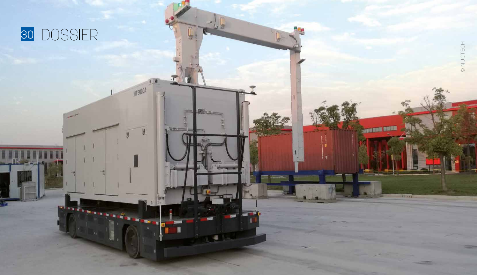
An NII system mounted on an automated guided vehicle
